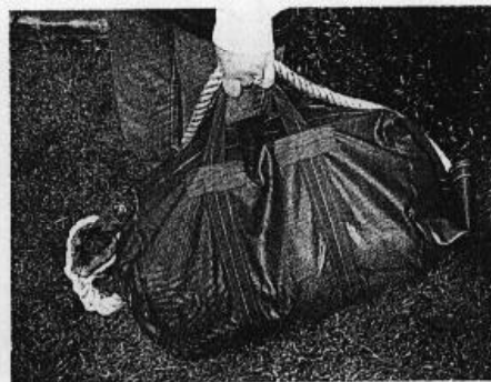
Specially designed rode bag - this one is 13x26in and holds 100m of 18mm line
