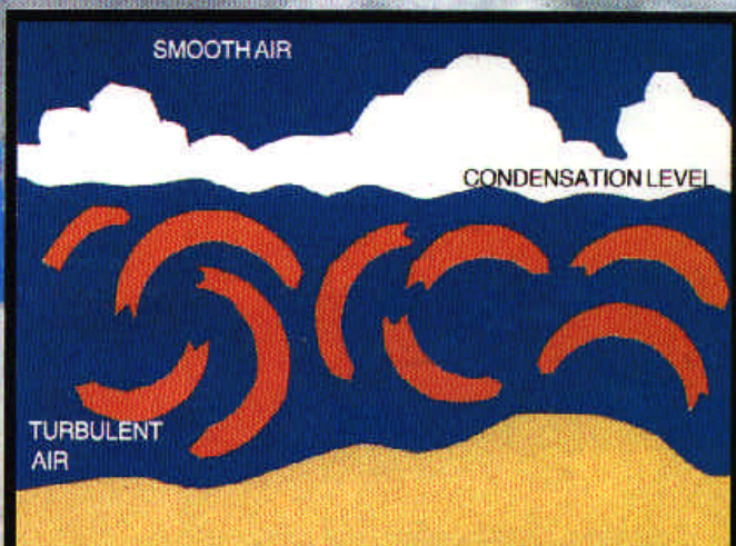
Mechanical (or frictional) turbulence occurs when the air flow is deformed into a series of eddies as it moves over the earth's surface.
